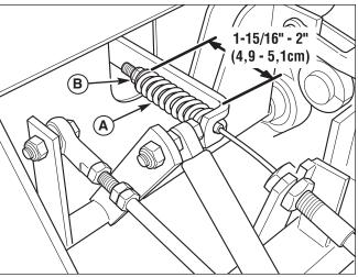
Figure 33. Parking Brake Adjustment
